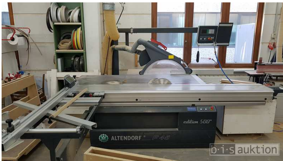
Formatkreissäge, Fabr. Altendorf, Typ F45/Edition 500 II, Bj. 2015 Format circular saw, manuf. Altendorf, model F45/edition 500II, made 2015
