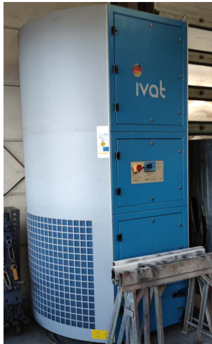
Schweißrauchabsaugung, Fabr. IVAT, Airtower 5000, Bj. 2019 weld smoke exhaust, Model IVAT airtower 5000, made 2019
